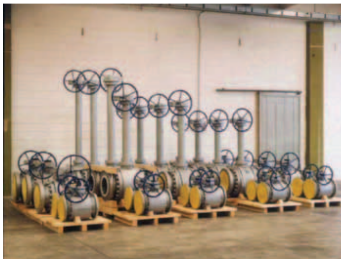
Misc. valves diam. underground extension
