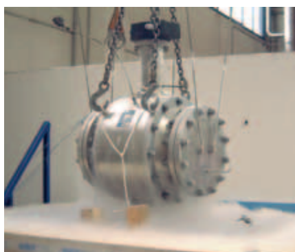
12" 150 class at cryo test
