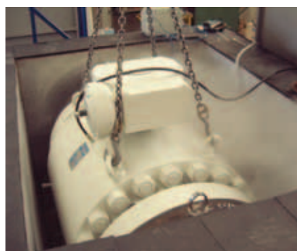
24" 900 class at low temp test
