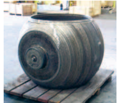
36" Ball overlayed in Alloy 625
